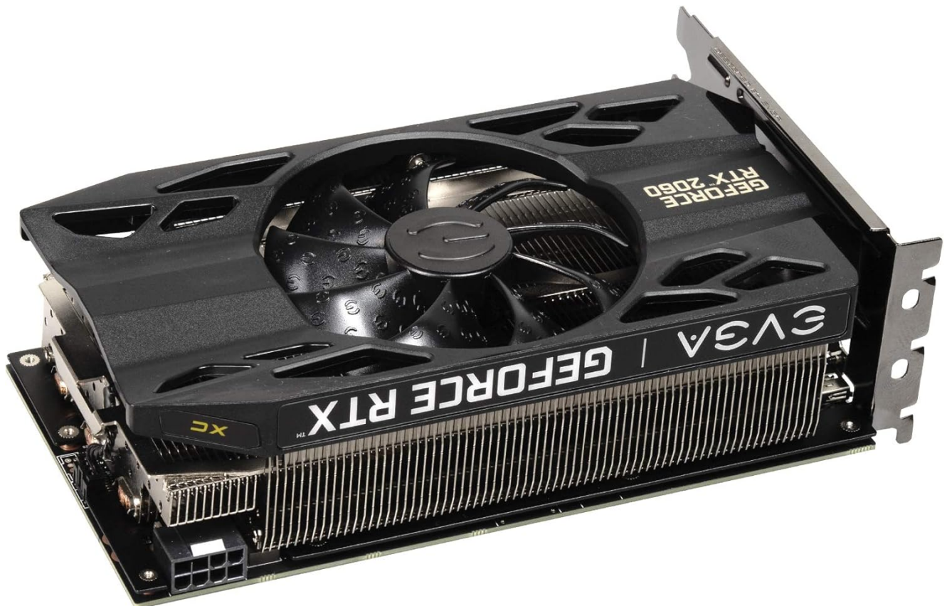
Image: Top view of the graphics card, highlighting the 8-pin PCIe power connector.
