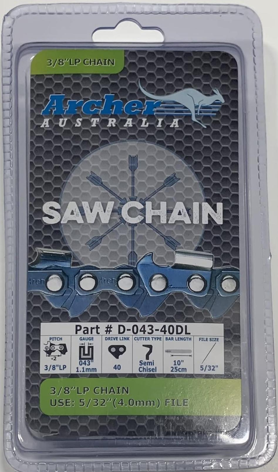
**Image 1.1:** Archer 10-inch Chainsaw Chain in its packaging. The label clearly displays the part number D-043-40DL, 3/8LP pitch, .043 gauge, 40 drive links, semi-chisel cutter type, 10-inch bar length, and recommended 5/32" (4.0mm) file size for sharpening.
