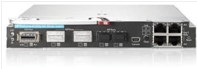
Figure 3.1: Front panel of the HP ProCurve 6120G/XG Blade Switch. This image displays the 10/100/1000 Ethernet ports, SFP ports, console port, and status indicators.
