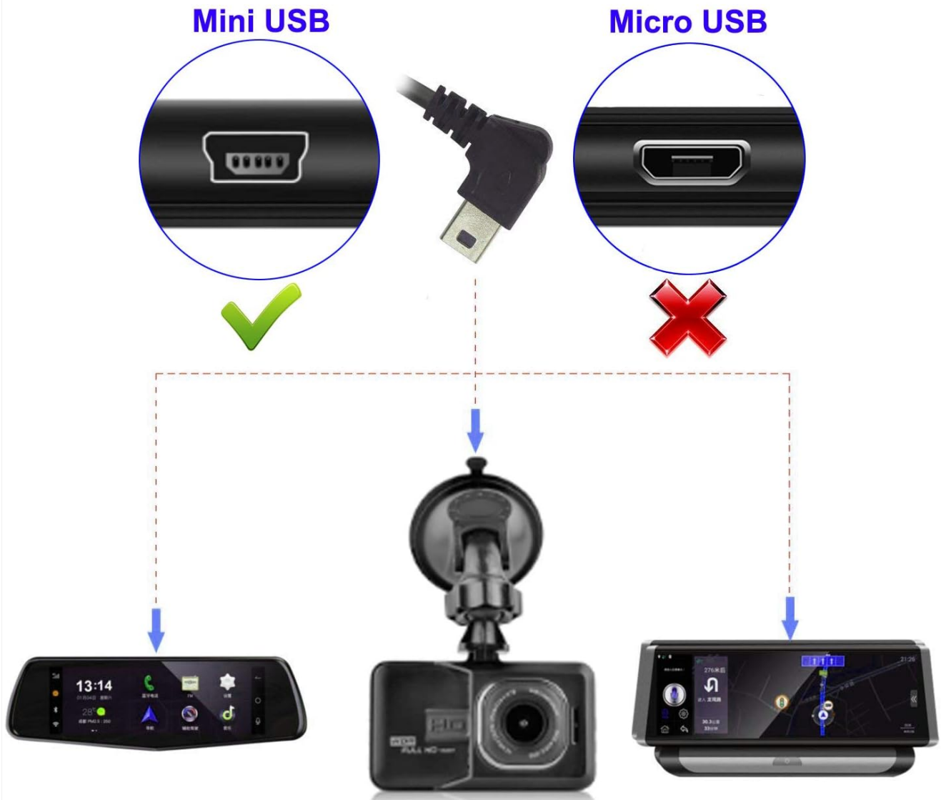
Image: Visual comparison of Mini USB (compatible) and Micro USB (incompatible) ports, highlighting the correct connector type for this kit.
