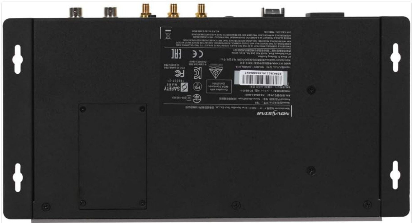
Figure 3.3: Rear panel of the Novastar TB3, detailing the various input/output ports, including antenna connectors, and regulatory labels.
