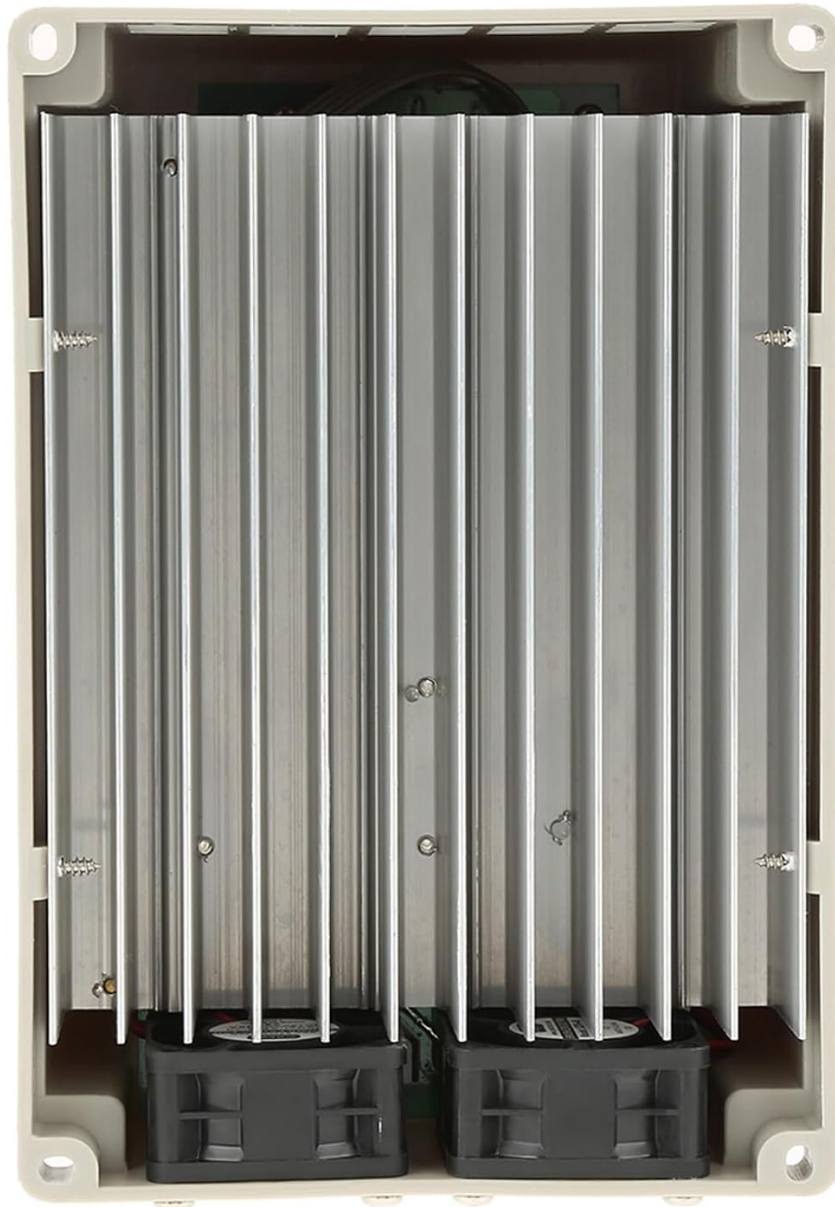
Figure 2: Internal view of the Hilitand AT1-2200X VFD, highlighting the large heatsink for efficient cooling.
