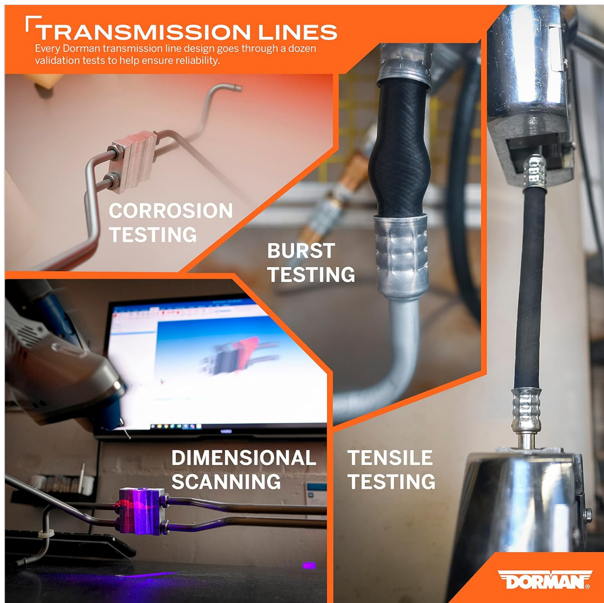
Image 2: Dorman's validation testing for transmission lines. This image illustrates various tests performed on transmission lines, including corrosion testing, burst testing, dimensional scanning, and tensile testing, ensuring product reliability.
