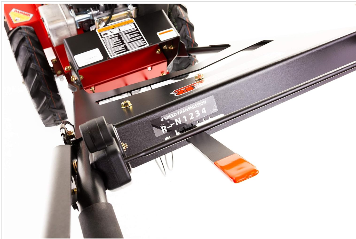
Figure 3: Detail of the 4-speed transmission lever with R-N-1-2-3-4 settings.
