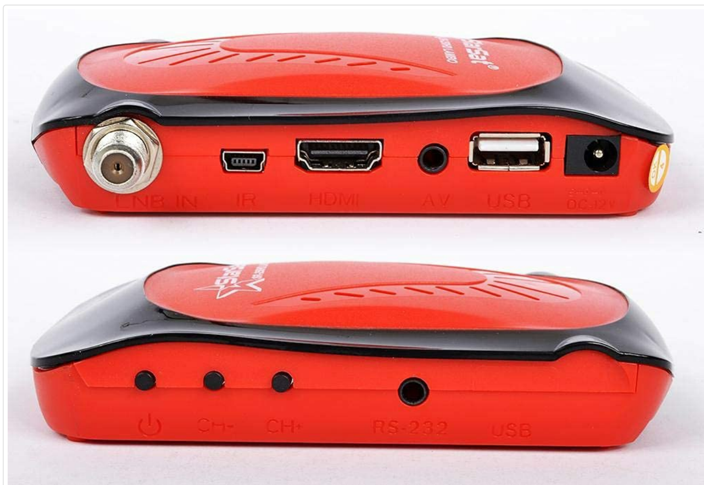
Image: Detailed view of the side panels showing all input/output ports and control buttons.
