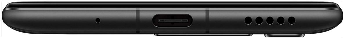
Figure 3.3: Bottom view of the HONOR View 20, showing the USB Type-C port for charging and data transfer.
