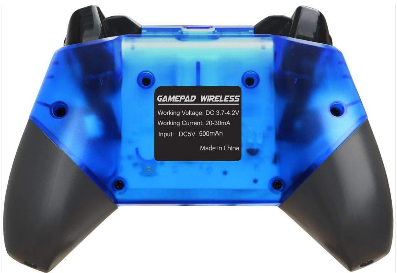
Image: Back view of the PAWHITS Wireless Pro Controller, displaying a label with technical specifications such as working voltage, current, and input.
