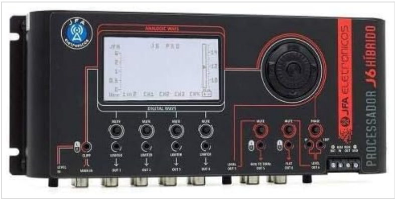
Figure 1: Front Panel View. This image displays the front panel of the JFA J6 Hybrid Digital Audio Processor. It features a central LCD screen for settings and monitoring, surrounded by a rotary encoder for navigation and adjustment. Below the screen are various buttons and indicators for input level, mute, limiter, and output level controls for each of the six channels. The 'LEVEL IN' and 'MAIN IN' indicators are visible on the left, while 'LEVEL OUT 5' and 'LEVEL OUT 6' are on the right, alongside the power terminal.
