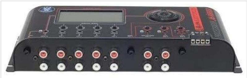
Figure 2: Rear Panel View. This image shows the rear panel of the JFA J6 Hybrid Digital Audio Processor, highlighting the input and output connections. On the left, there are RCA input jacks labeled 'MAIN IN'. The center features multiple RCA output jacks for OUT 1 through OUT 6. On the right, a screw terminal block is visible for power connections (BAT, REM, GND).
