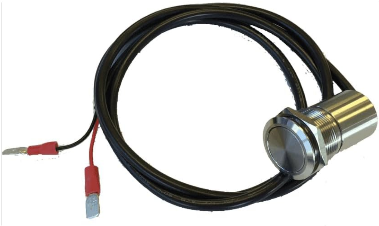
Figure 3.2: Angled view of the Lowrance AUTO-STBY Button Metal, highlighting the threaded body and securing nut, indicating its panel-mount design.
