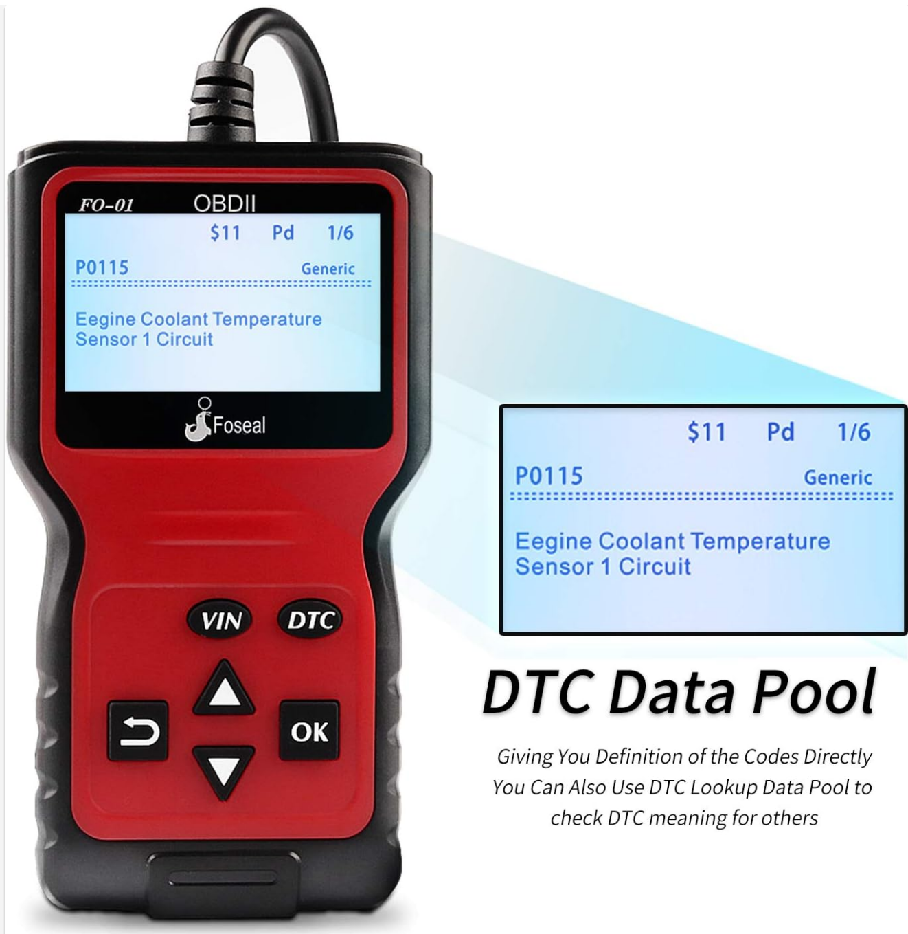
Figure 5: The FO-01 displaying a Diagnostic Trouble Code (DTC) and its corresponding definition.
