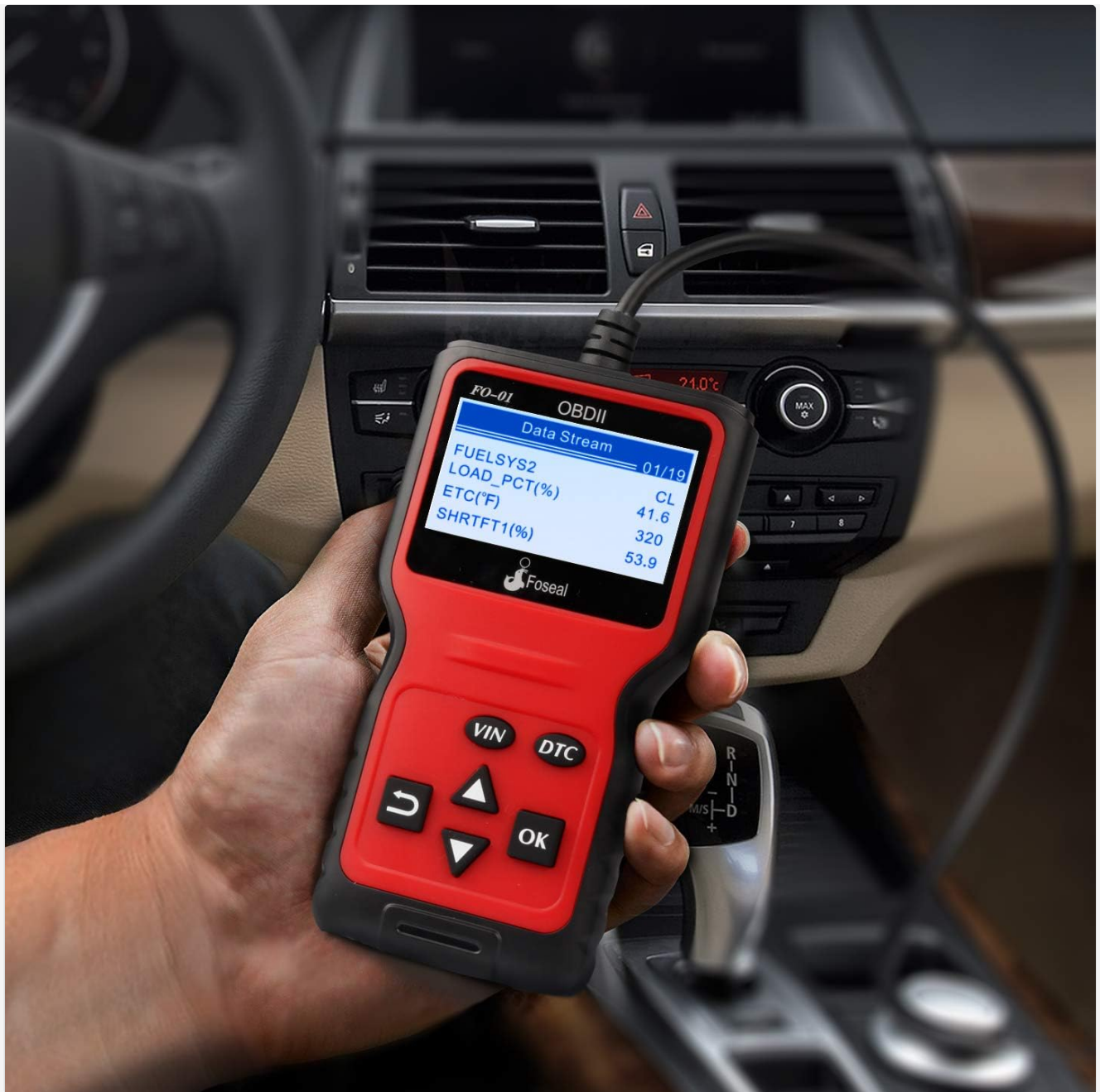
Figure 4: The Foseal FO-01 connected to a vehicle's OBDII port, displaying live data.
