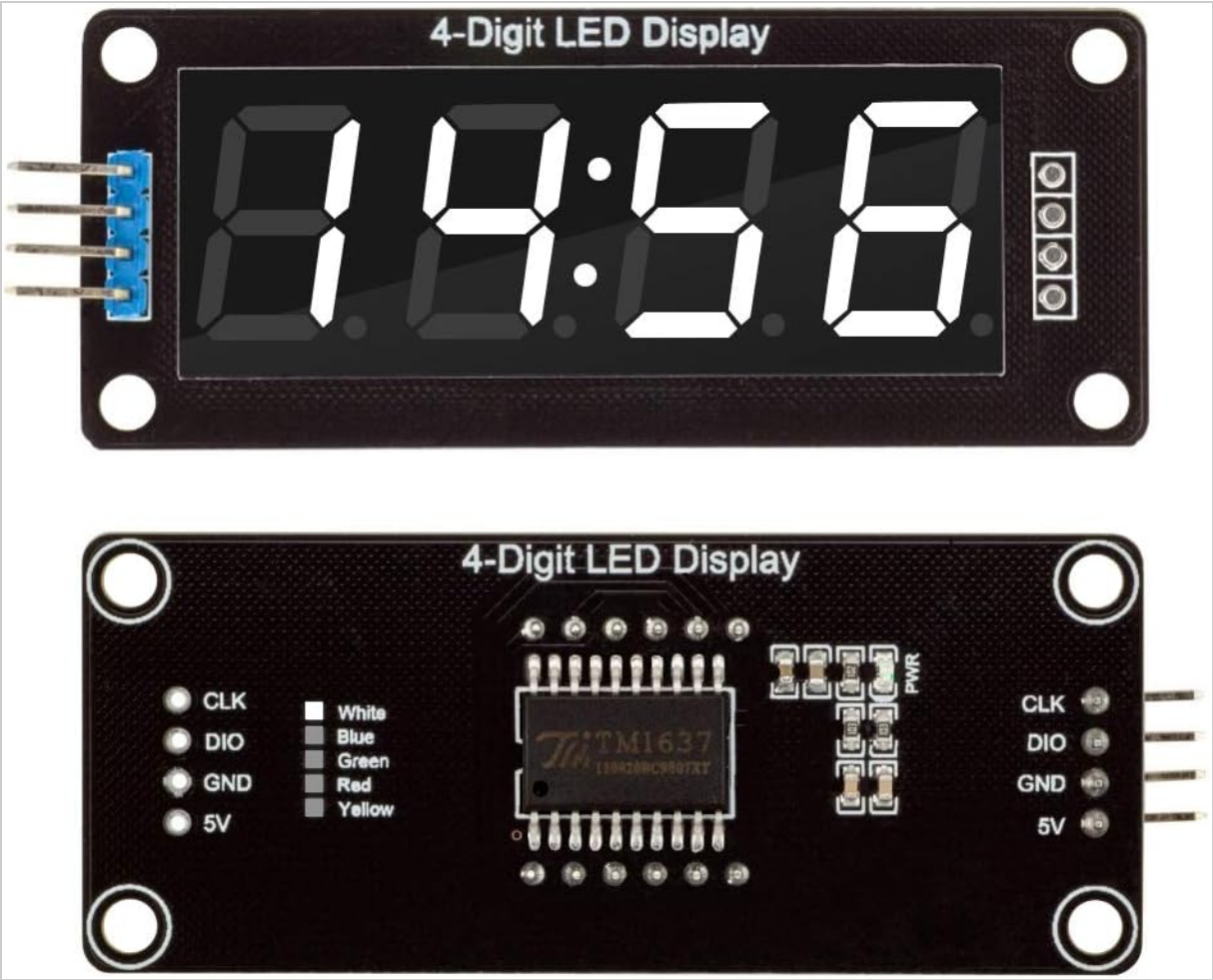
Image: Front and back views of a white diymore TM1637 module, illustrating the display and the pin connections on the reverse side, ready for integration into a circuit.
