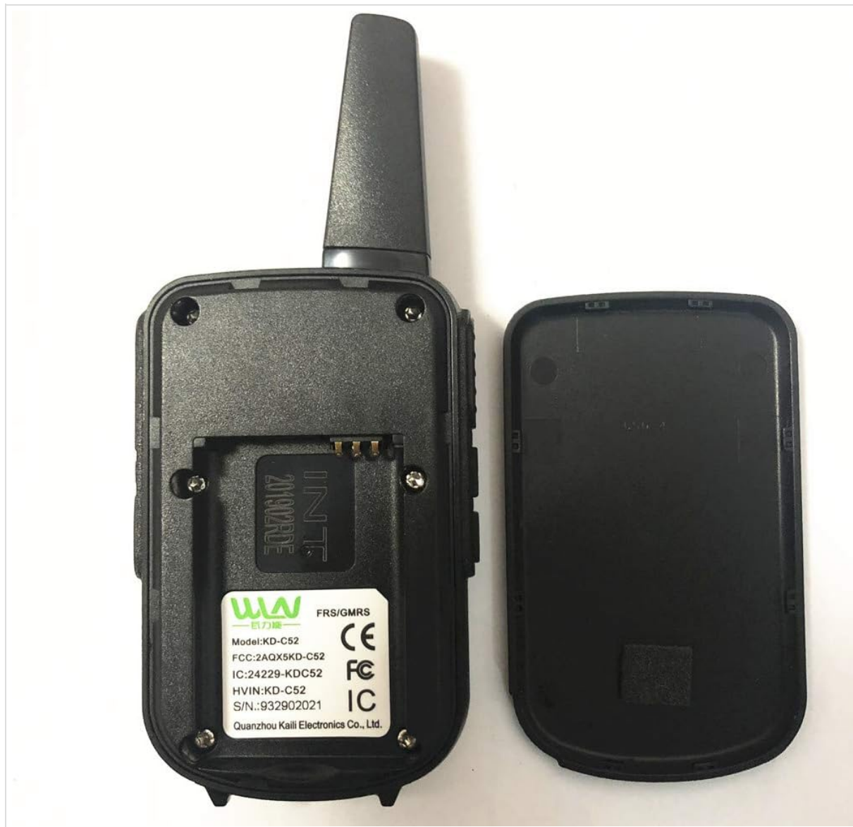
Image: The back view of the WLN KD-C52 Walkie Talkie with the battery compartment cover removed, showing the battery slot and regulatory information labels.
