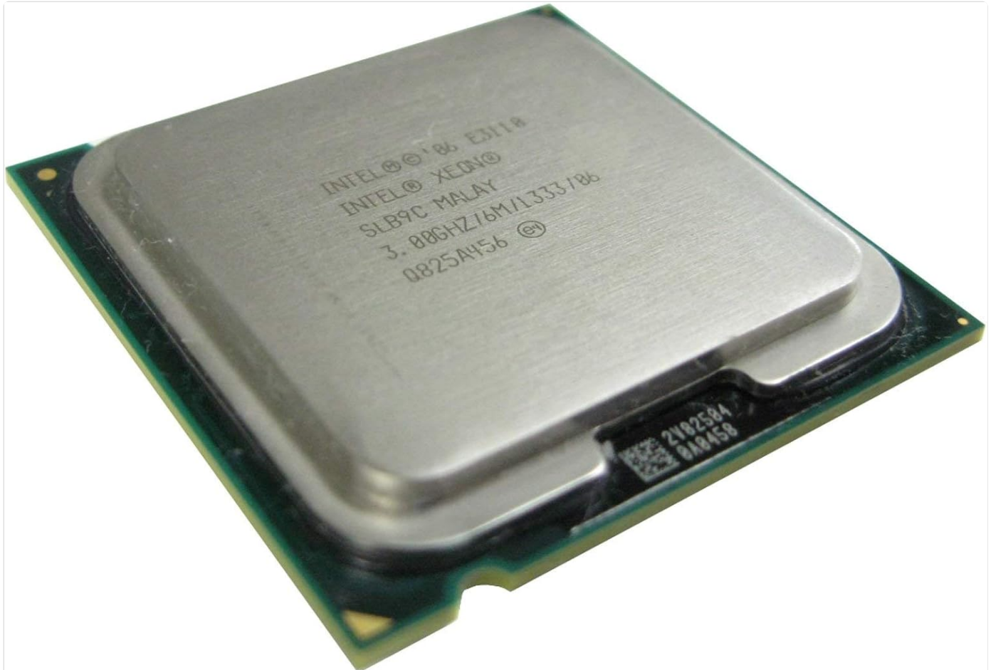
Figure 1.1: Top view of the Intel Xeon E3110 processor, showing the integrated heat spreader (IHS) with Intel branding and model information.
