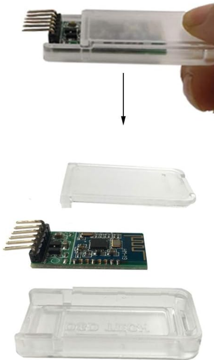
Image 7: The HM-19 module being inserted into a clear protective casing. This demonstrates how the module can be protected from environmental factors.
