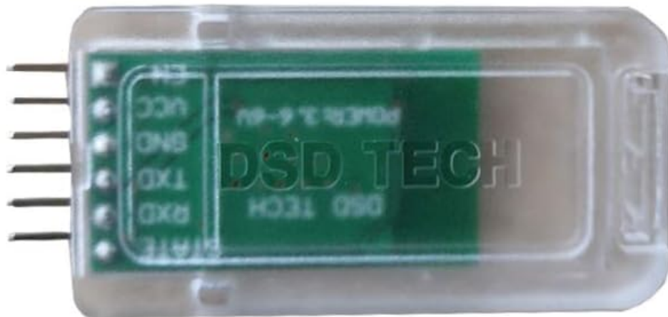
Image 8: Top and bottom views of the HM-19 module fully enclosed in its protective casing. This shows the module's appearance when housed, with pins exposed for connection.
