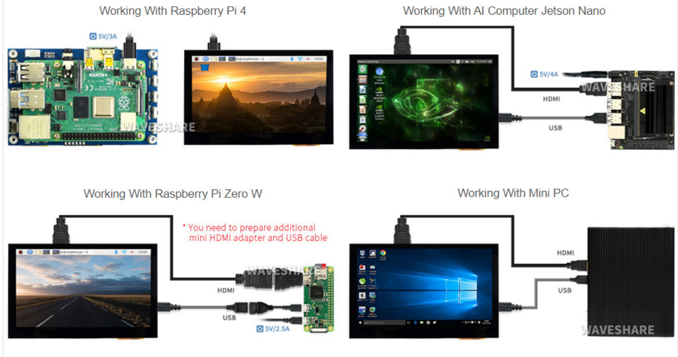
Image: Visual examples of connecting the display to Raspberry Pi 4, Raspberry Pi Zero W, Jetson Nano, and a Mini PC.
