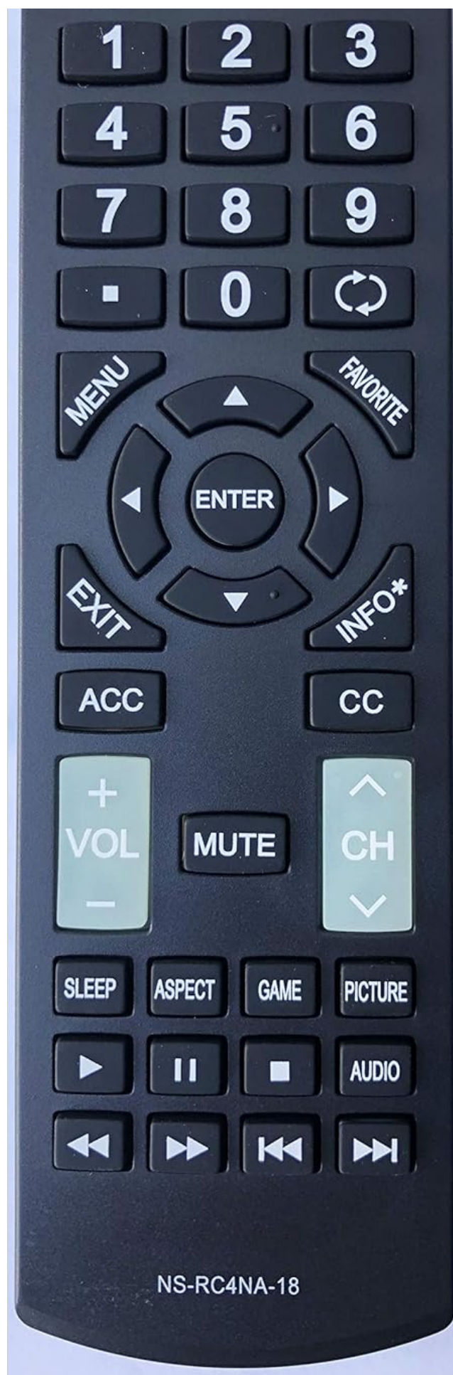
Figure 2.1: Front view of the NS-RC4NA-18 remote control. The battery compartment is located on the reverse side.
