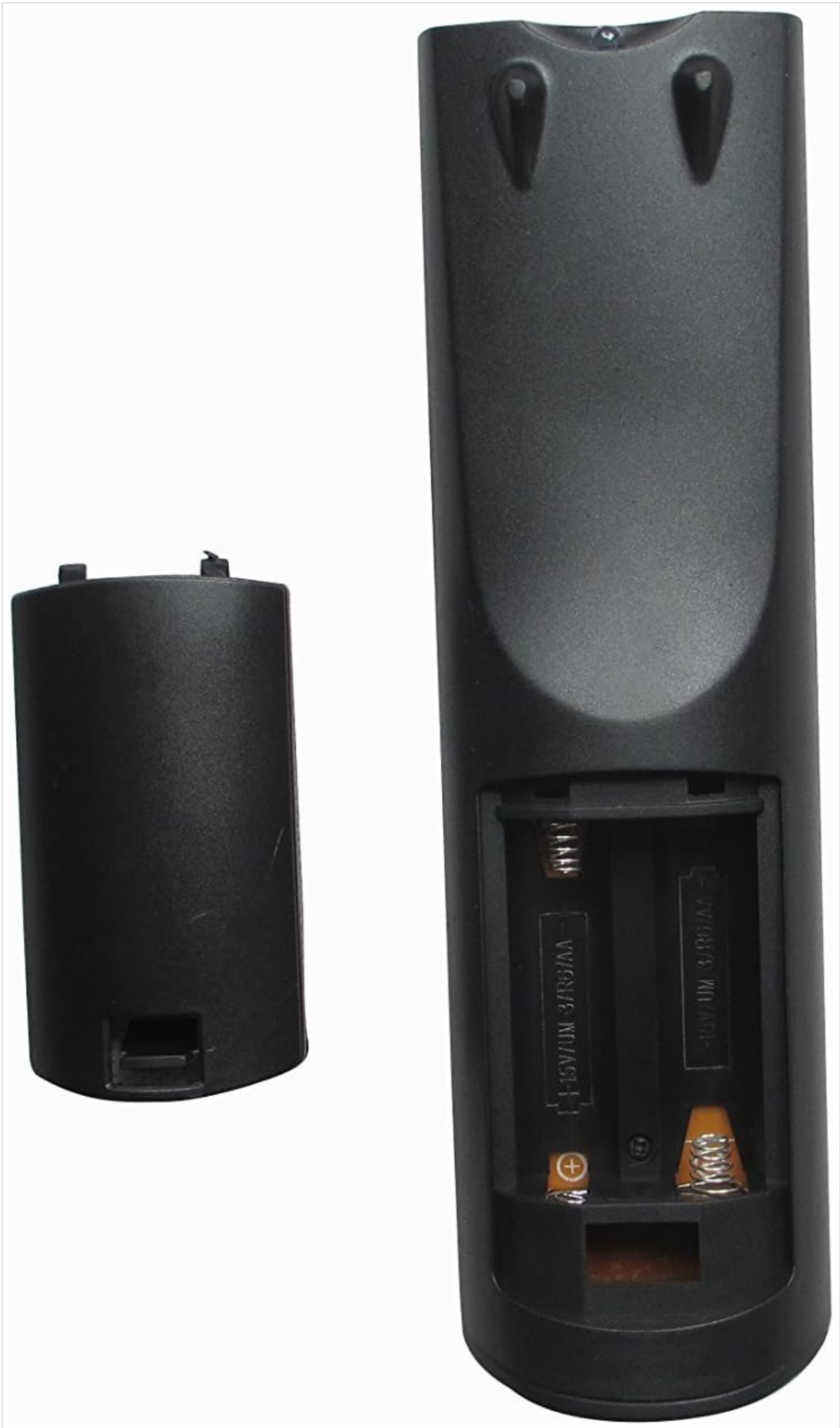
Figure 1: Battery compartment with cover removed, showing where to insert two AA batteries.
