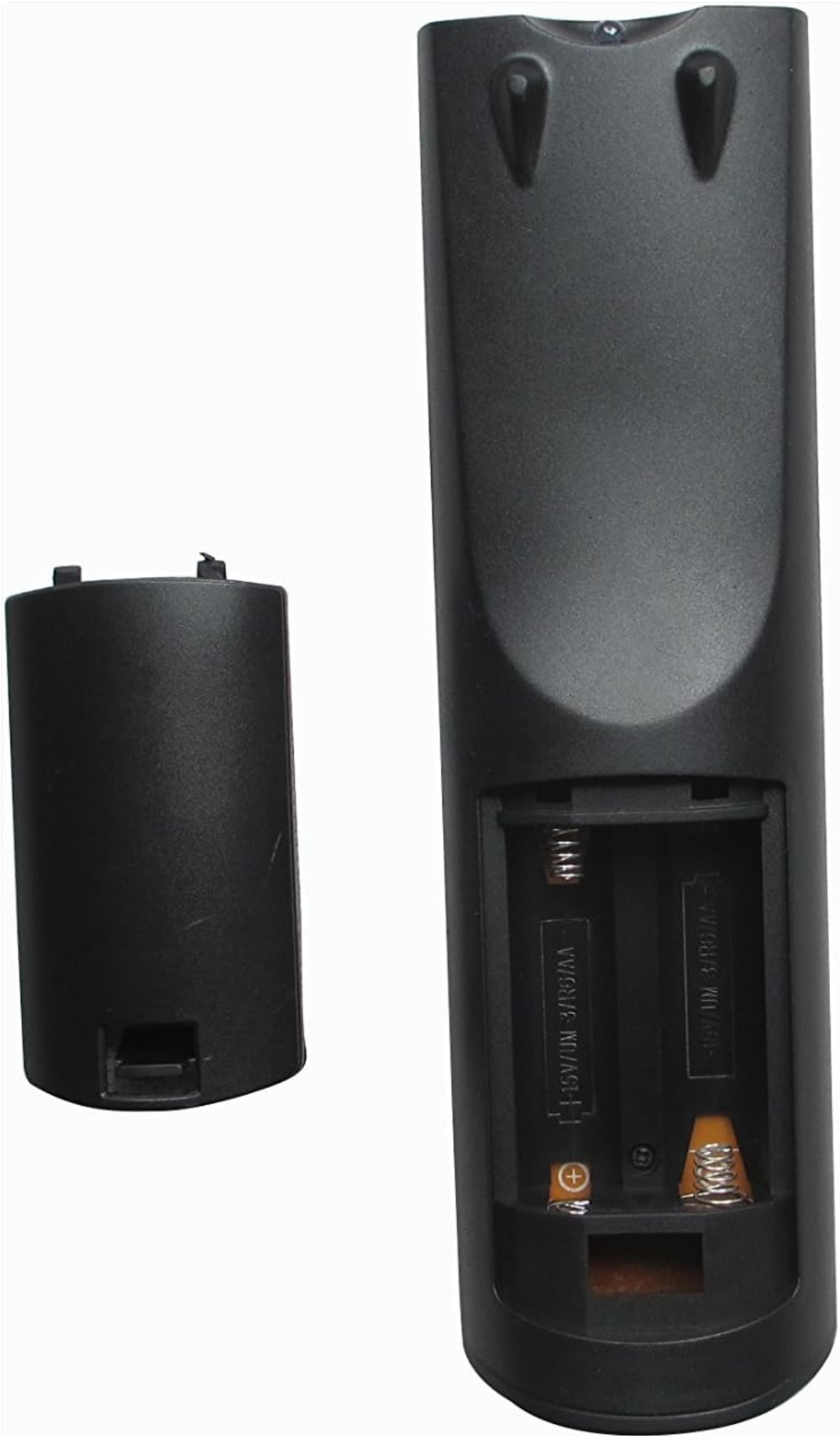
Image 2: Another perspective of the remote control's rear, with the battery cover removed, clearly showing the two AA
