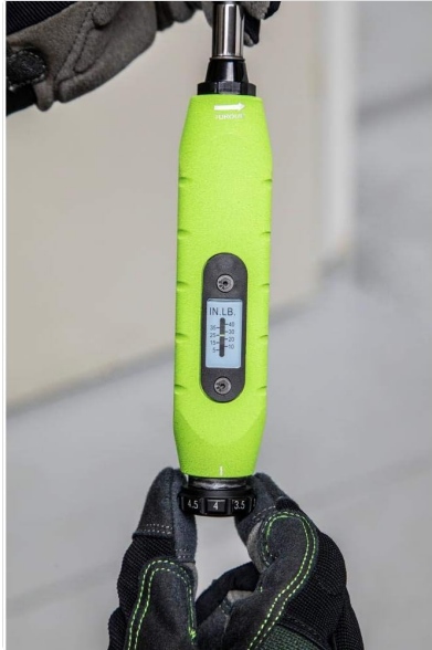
Figure 2: Hands adjusting the torque setting on the Greenlee 0153-46T. This image illustrates the bottom adjustment dial and the torque scale on the side of the tool, demonstrating how users interact with the device to set the desired torque.
