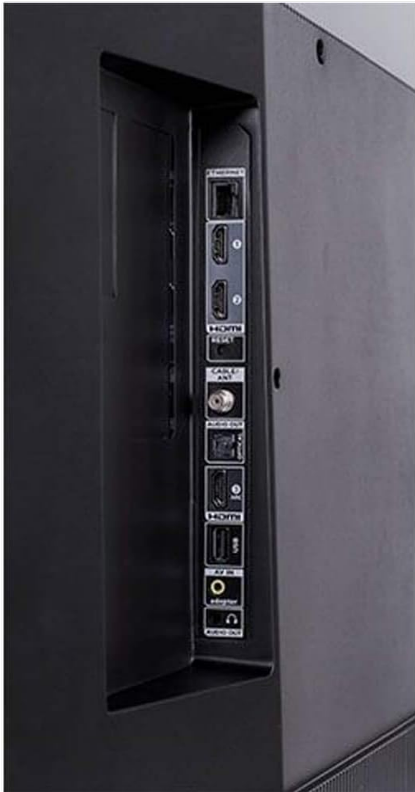
Image: A detailed view of the input ports on the back of the TCL TV, including HDMI, USB, and AV inputs.
