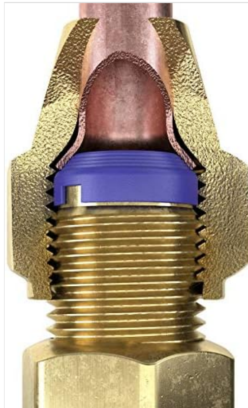
Figure 3.3: Cross-section illustrating the FlareSeal compressed within a tightened flare connection, ensuring a leak-free seal.
