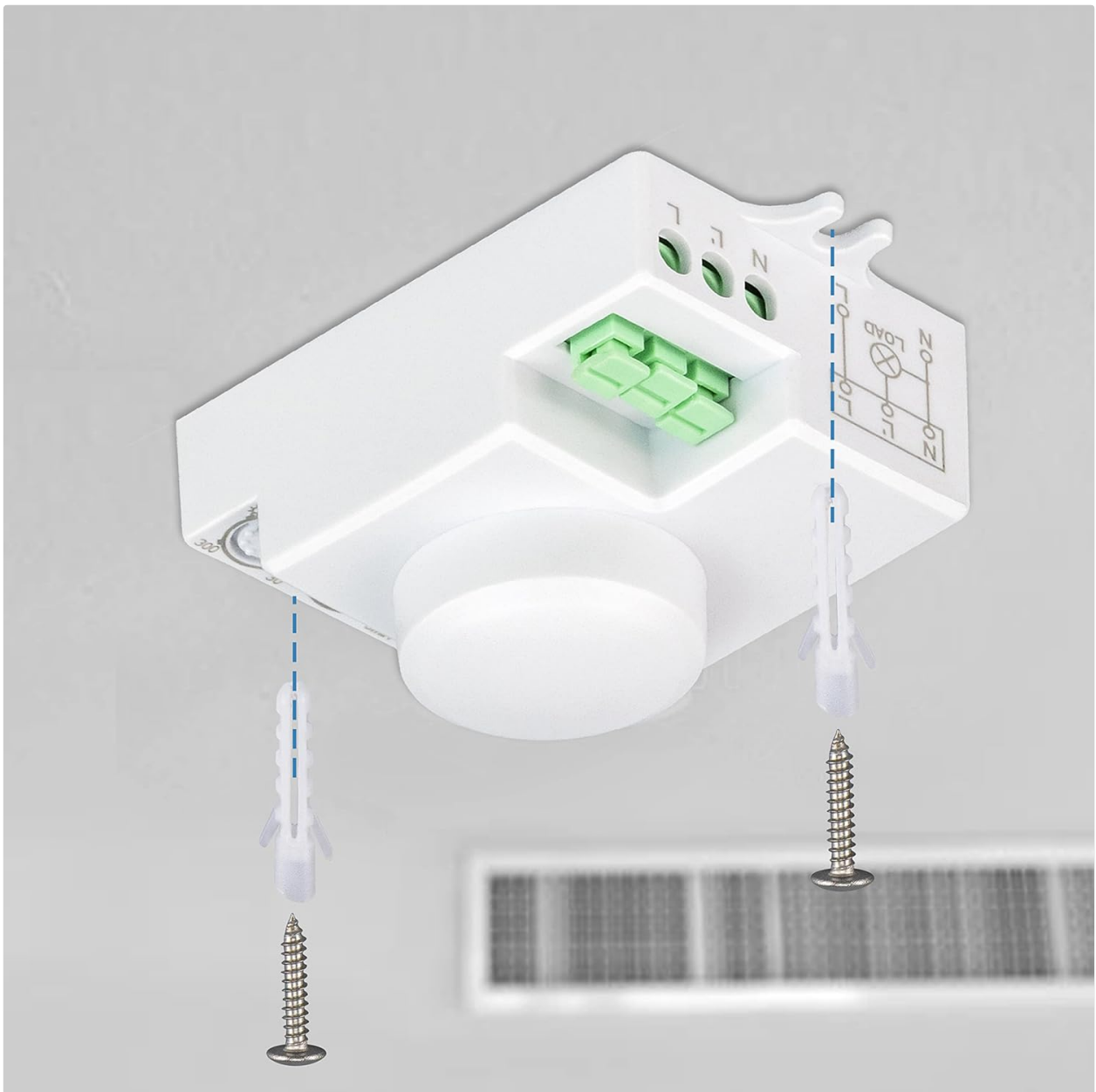
Figure 5.1: Wiring connections for the POPP SM-001 sensor. Connect the Live (L), Neutral (N), and Load (L') wires as indicated. The load is the light fixture or device to be controlled.
