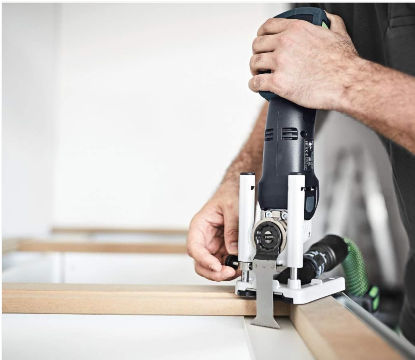
Figure 5.2: Demonstrating the tool's capability for plunge cuts, possibly for creating openings in panels or for precise trimming.
