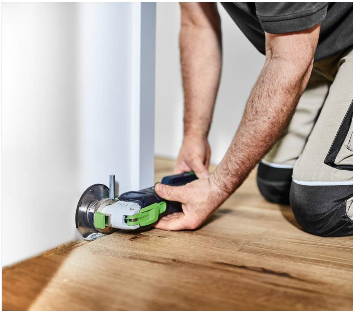
Figure 5.5: The multi-tool being used for a precise flush cut, demonstrating its ability to trim materials close to a surface, such as a door frame or baseboard.
