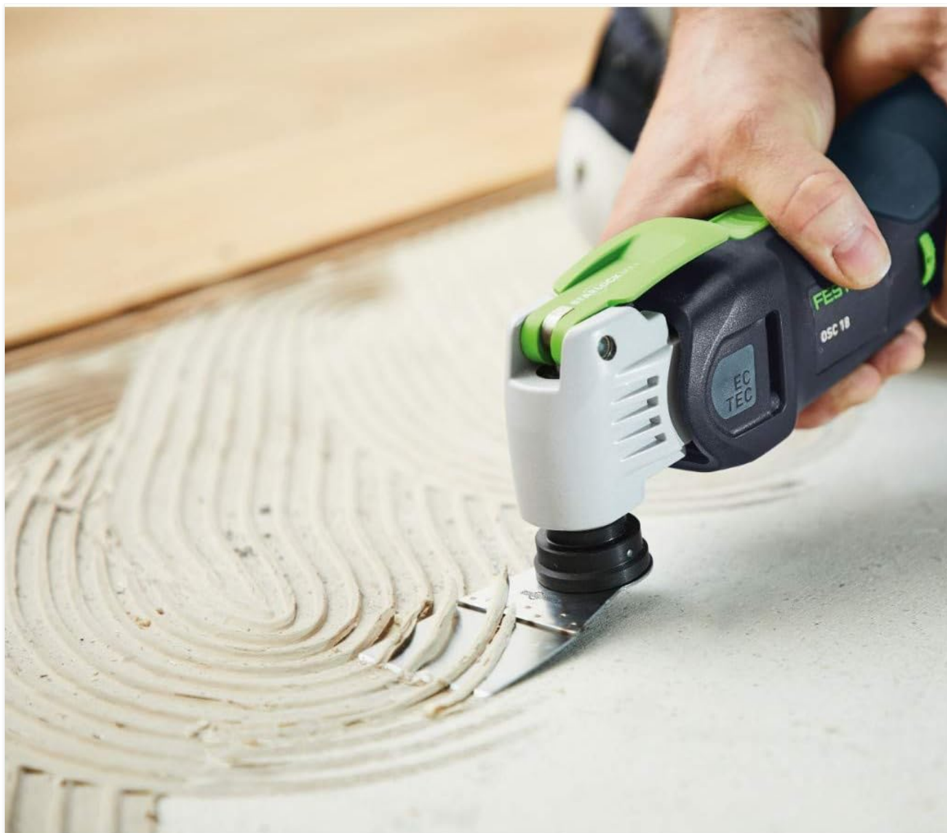
Figure 5.3: The multi-tool equipped with a scraper blade, effectively removing dried adhesive or similar material from a surface.
