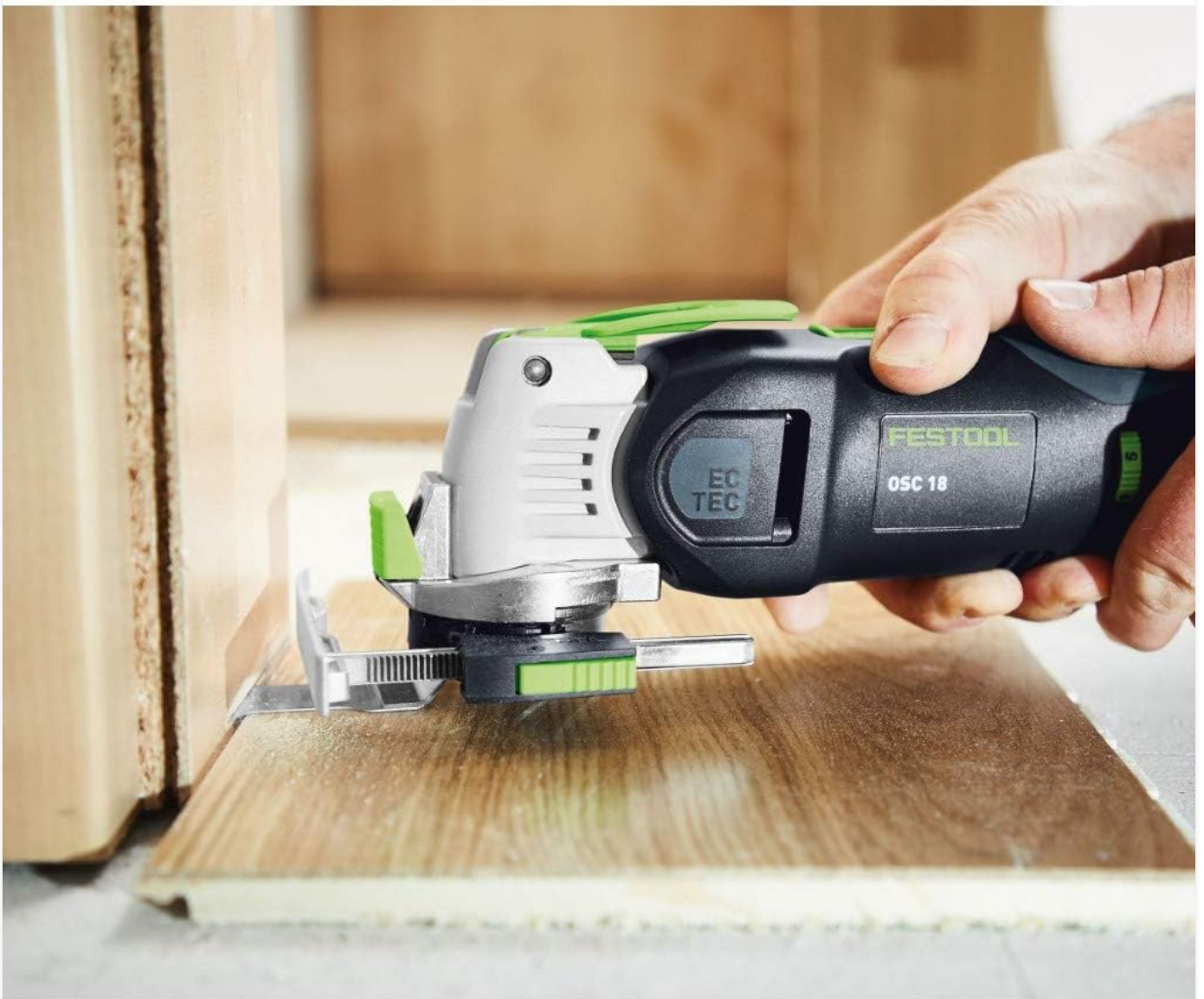
Figure 5.1: The multi-tool in action, demonstrating precise cutting of wood flooring, ideal for fitting around door frames or other obstacles.
