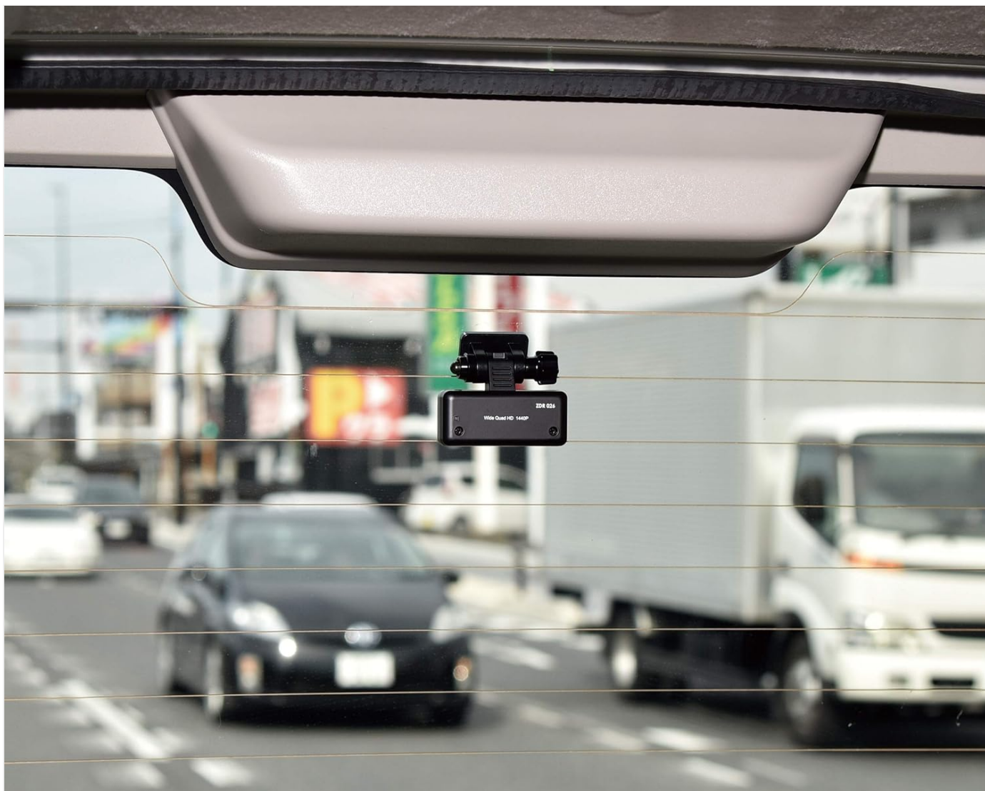
Image: The rear camera of the drive recorder installed on the rear window, showing the view of traffic behind.
