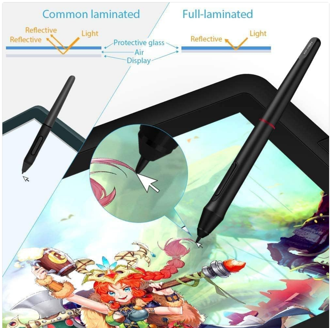
Image 4.4: A visual comparison illustrating the benefits of full-laminated technology in reducing the gap between the pen tip and the cursor, enhancing precision.
