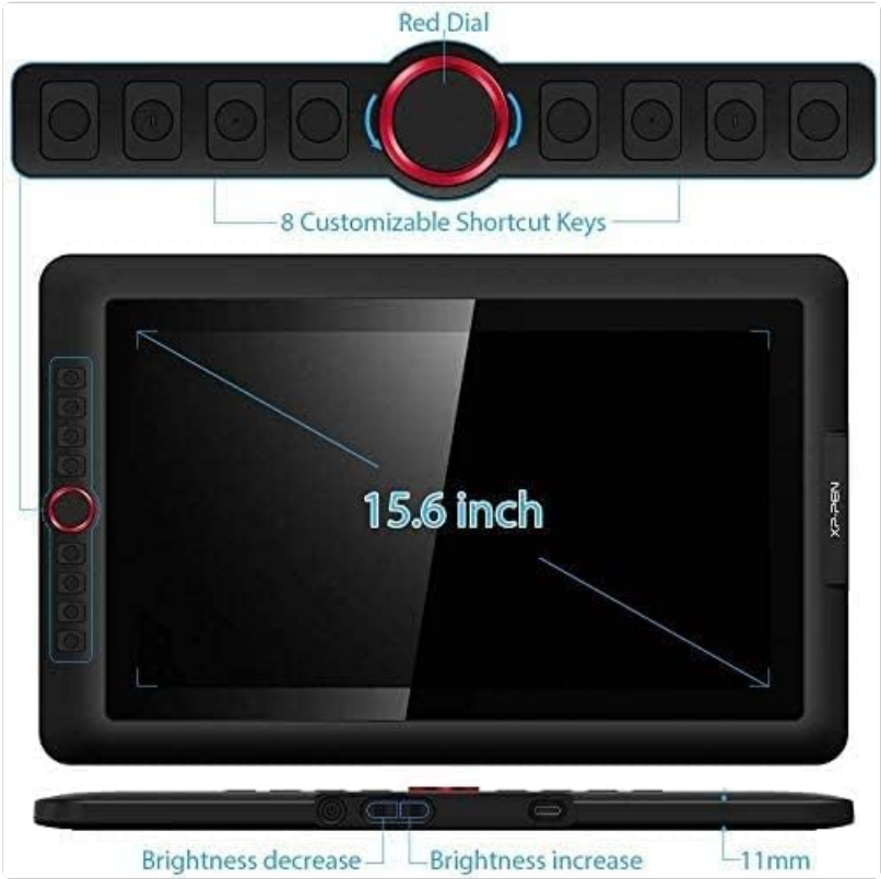
Image 4.1: The side profile of the Artist 15.6 Pro, highlighting the power button and brightness controls.
