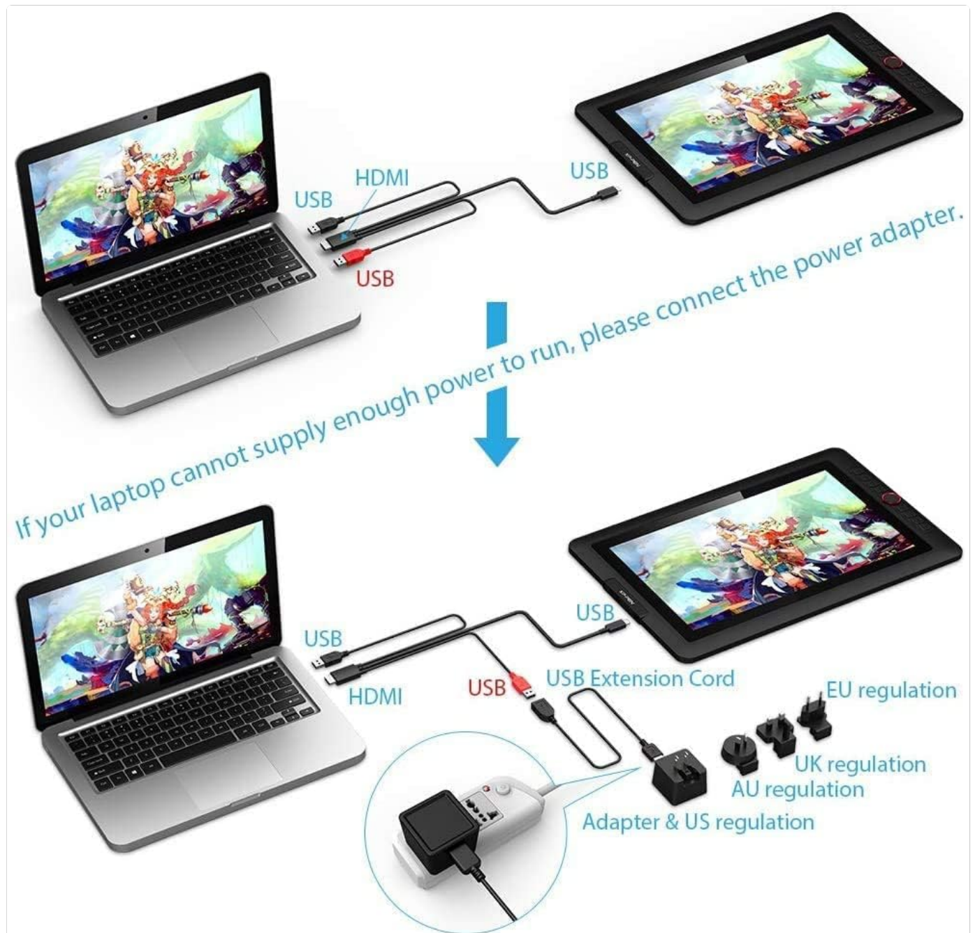
Image 3.1: Connection diagram for the Artist 15.6 Pro, illustrating the 3-in-1 cable setup with a laptop and external power.
