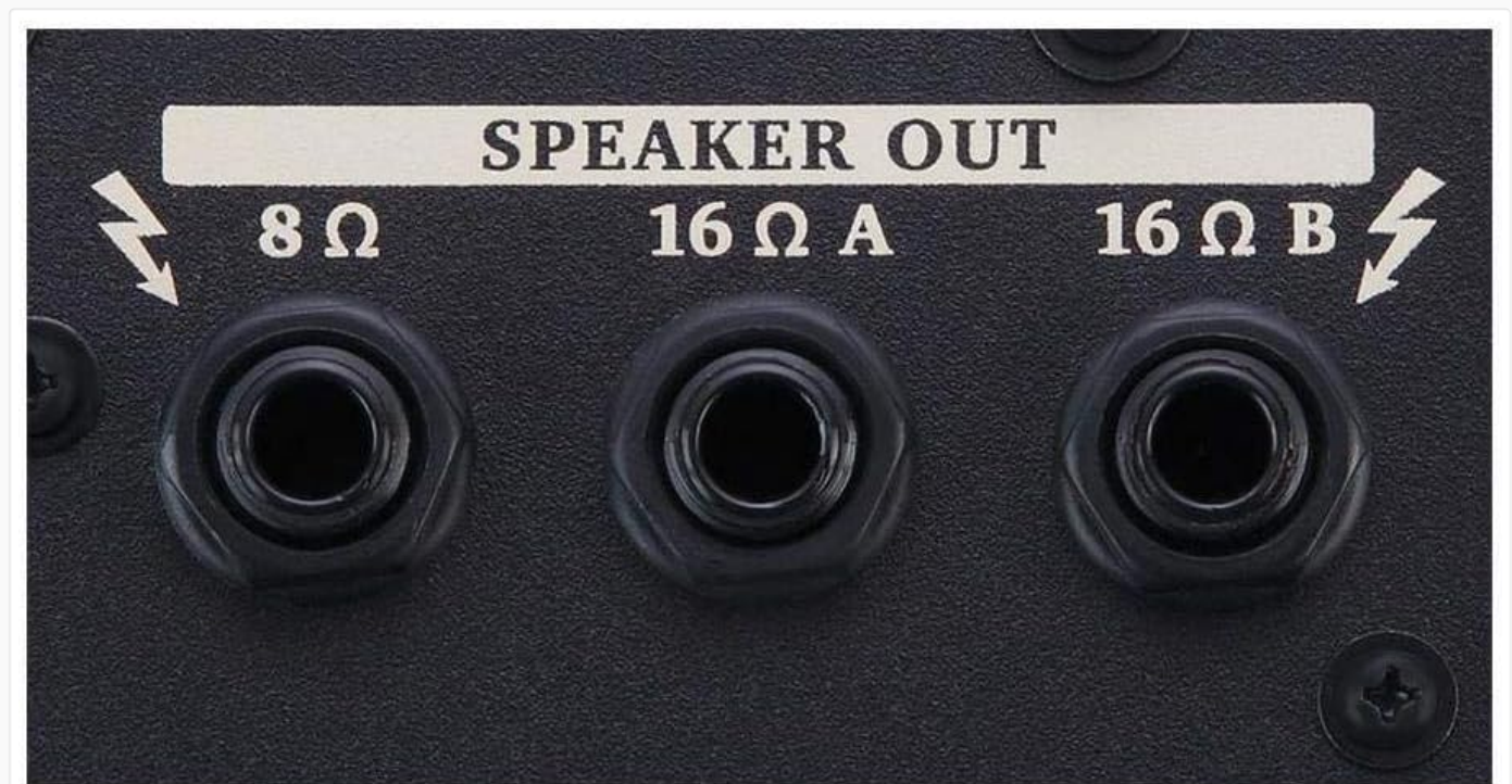
Figure 4: Speaker output jacks (8Ω, 16Ω A, 16Ω B) on the rear panel.
