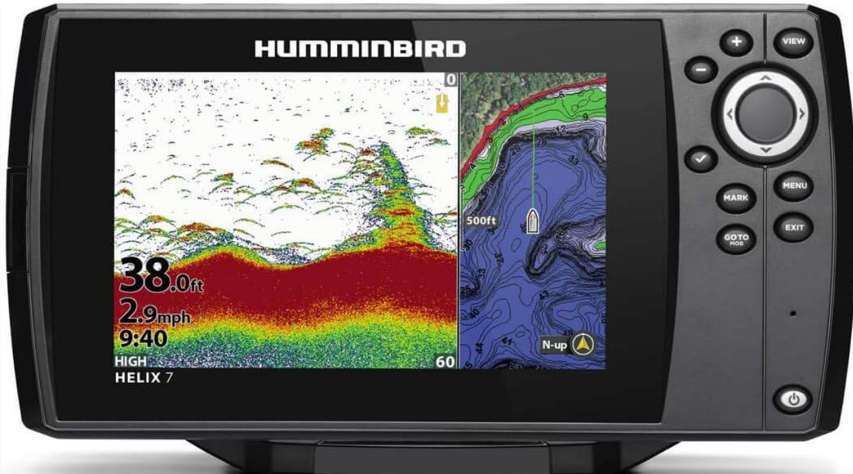
This image captures the Helix 7's display showing a vibrant sonar return. Clear fish arches are visible, indicating the presence of fish, along with detailed representations of the bottom structure and vegetation.
