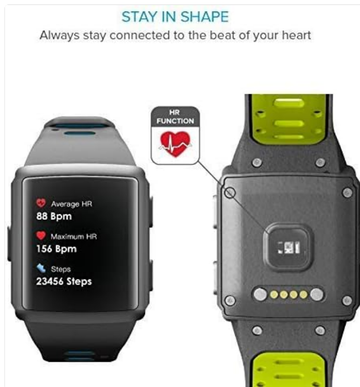
Figure 3.3: Rear view of the smartwatch, illustrating the integrated heart rate (HR) sensor designed for continuous monitoring during activities.
