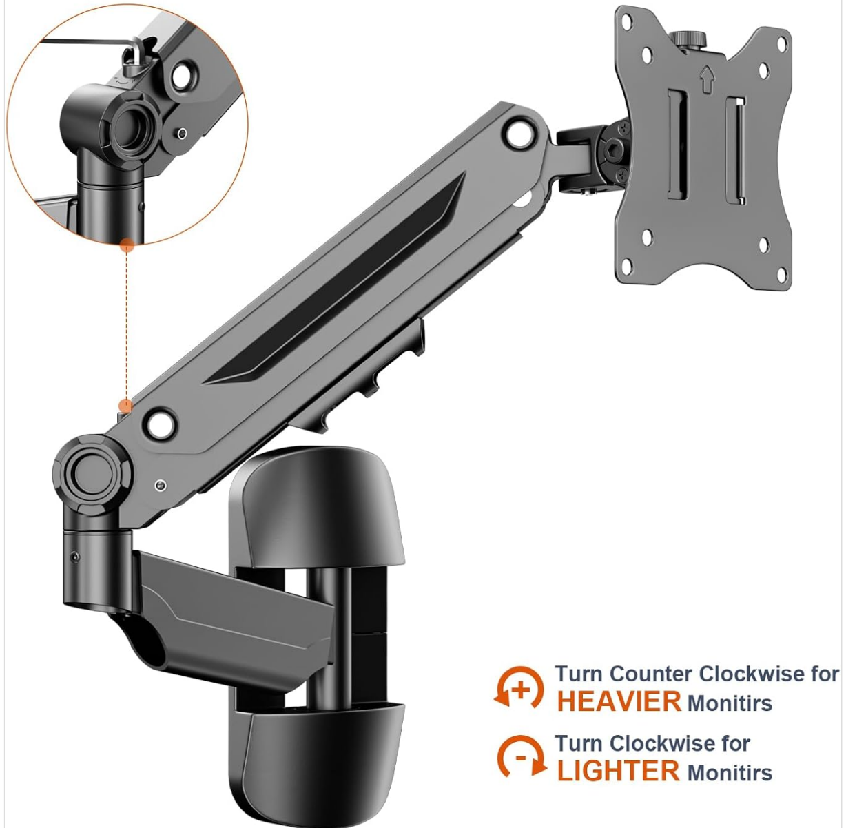
Figure 4: Gas Spring Tension Adjustment. This diagram shows the adjustment point on the arm and indicates turning counter-clockwise for heavier monitors (+) and clockwise for lighter monitors (-).
