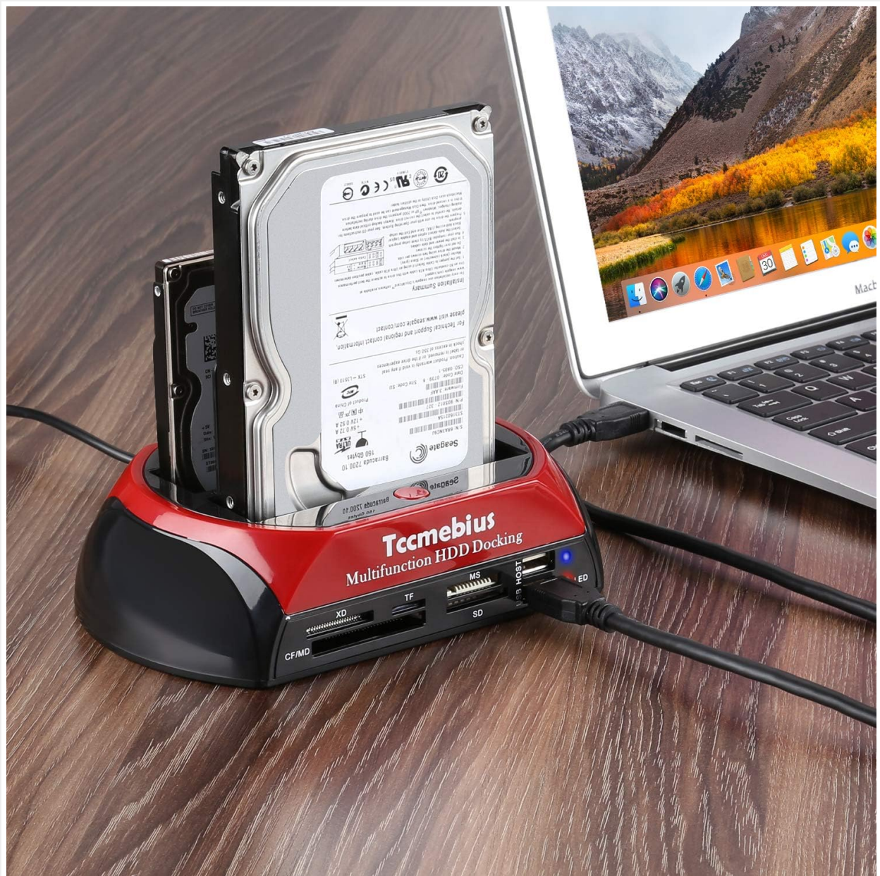
Figure 6: Docking station with hard drives connected to a computer.
