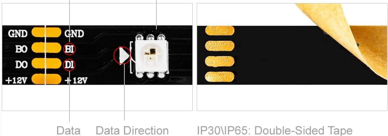
Image 2.1: Illustration of WS2815 dual signal break-point continuous transmission, where a defective LED does not stop the signal for subsequent LEDs.
