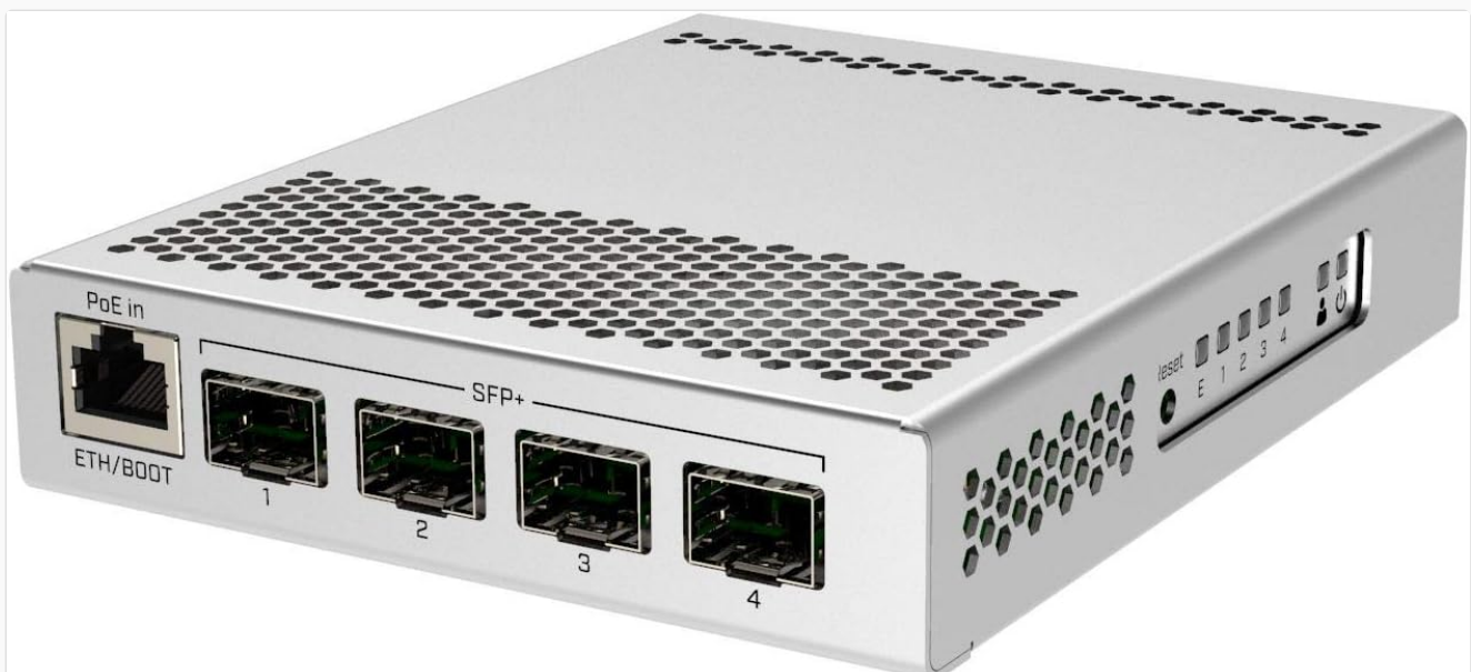
Figure 1: Front-top view of the MikroTik CRS305-1G-4S+in Network Switch, showing the Ethernet port and four SFP+ ports.
