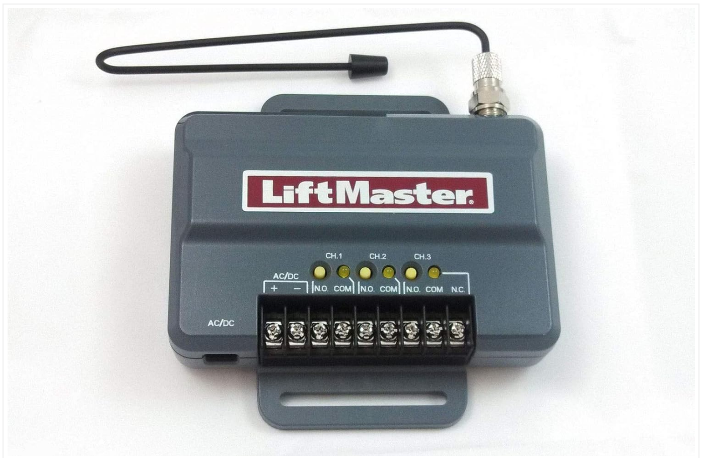
Figure 2: The LiftMaster 850LM Universal Receiver showing its terminal block for wiring connections and the antenna port. Labels for AC/DC power input and three channels (CH.1, CH.2, CH.3) with N.O., COM, N.C. contacts are visible.
