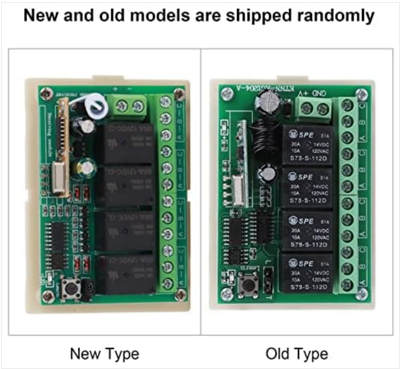
Figure 2.2: Comparison of two versions of the KG1204-A receiver circuit board, labeled "New Type" and "Old Type". Both show similar components and terminal layouts, indicating functional equivalence despite minor design variations.
