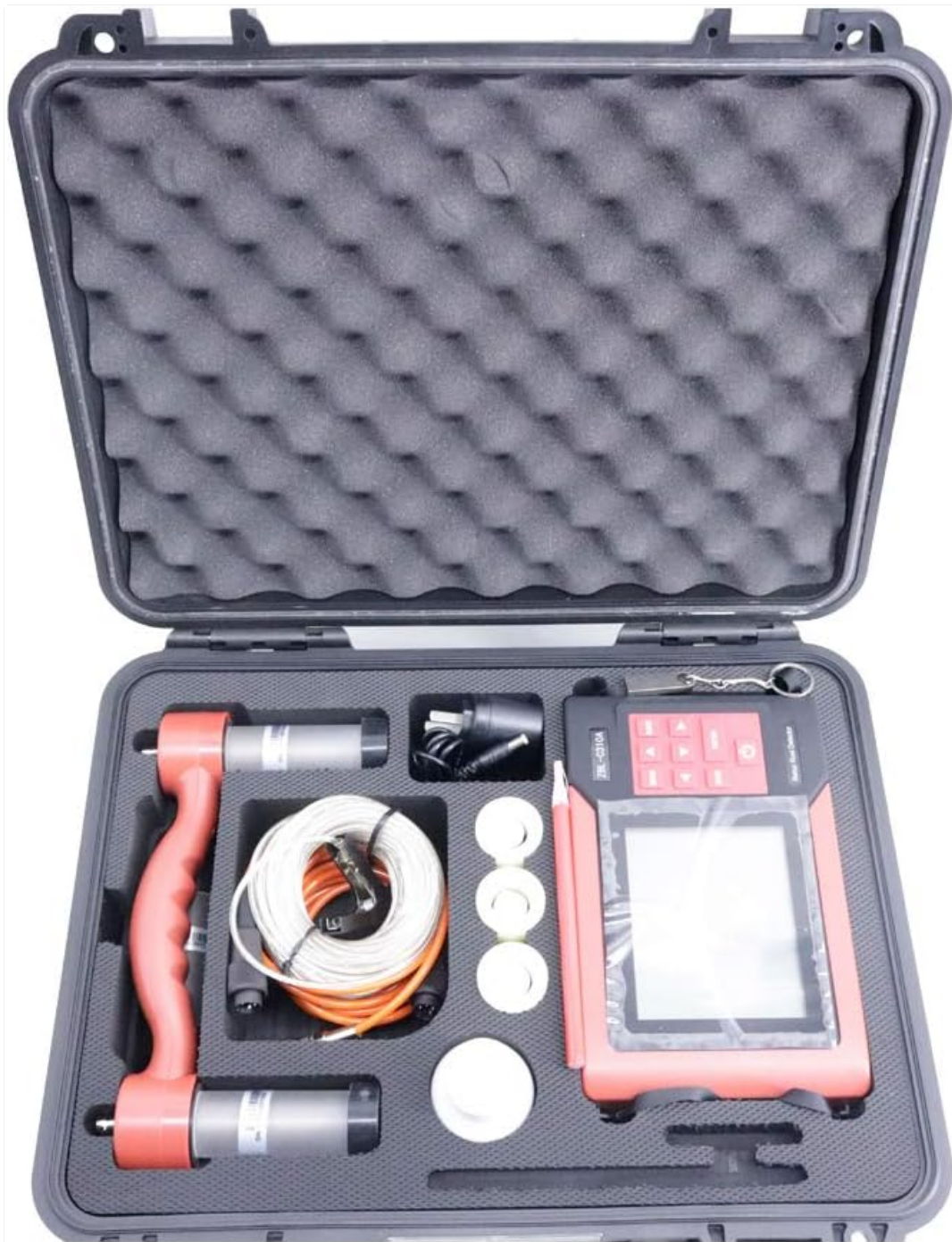
Figure 2.1: Complete ZBL-C310A kit in its protective carrying case, showing the main unit, probes, cables, and accessories neatly organized.
