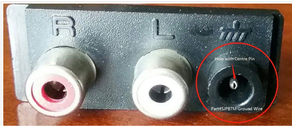
Image 2: Example of a turntable's ground wire receptacle. The image highlights the specific ground hole with a visible center pin, which is required for compatibility with this ground wire.
