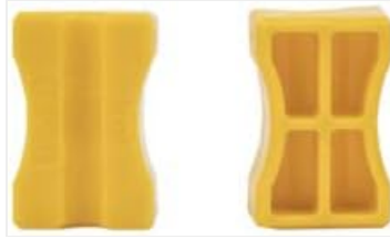
Image 3.5: Yellow brake pad spacers. These are typically used to prevent the brake pads from closing when the wheel or rotor is removed, protecting the hydraulic system.
