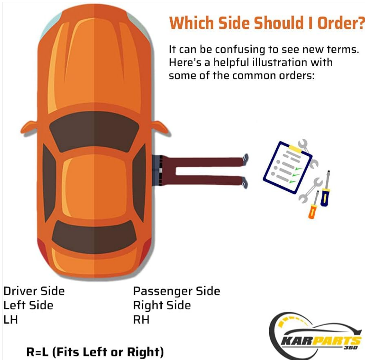
Figure 2: Diagram explaining vehicle side orientation. The 'Driver Side' refers to the left side of the vehicle when seated in the driver's seat, also known as LH (Left Hand).
