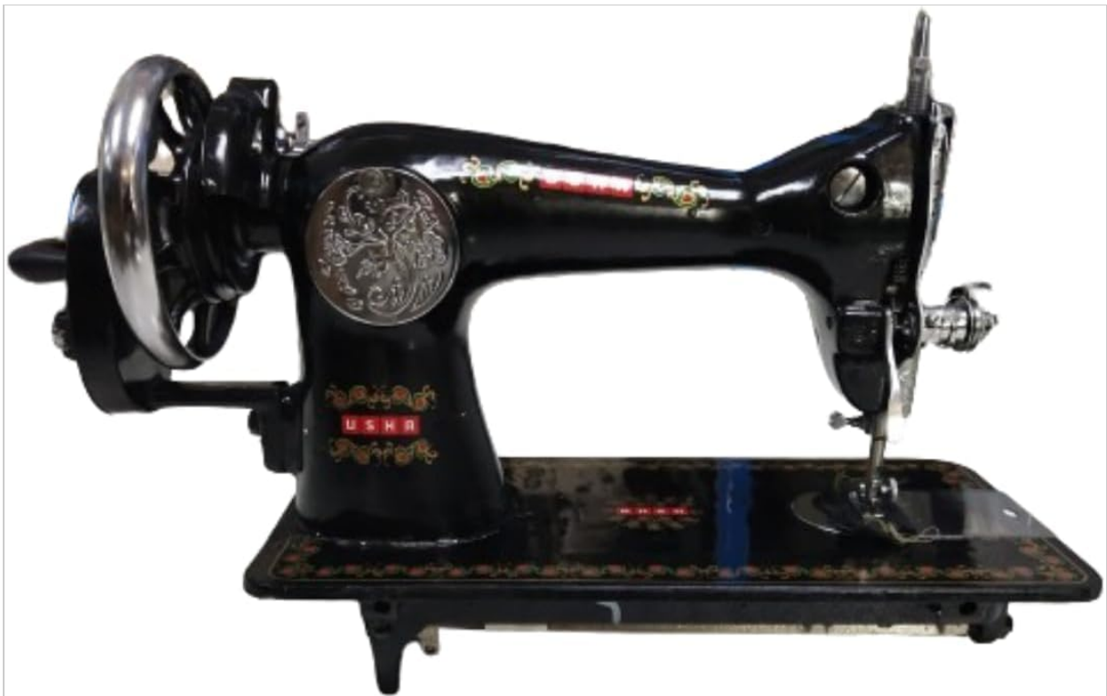
Figure 2: Side view of the USHA Ayush Sewing Machine, highlighting the hand crank and flywheel.
