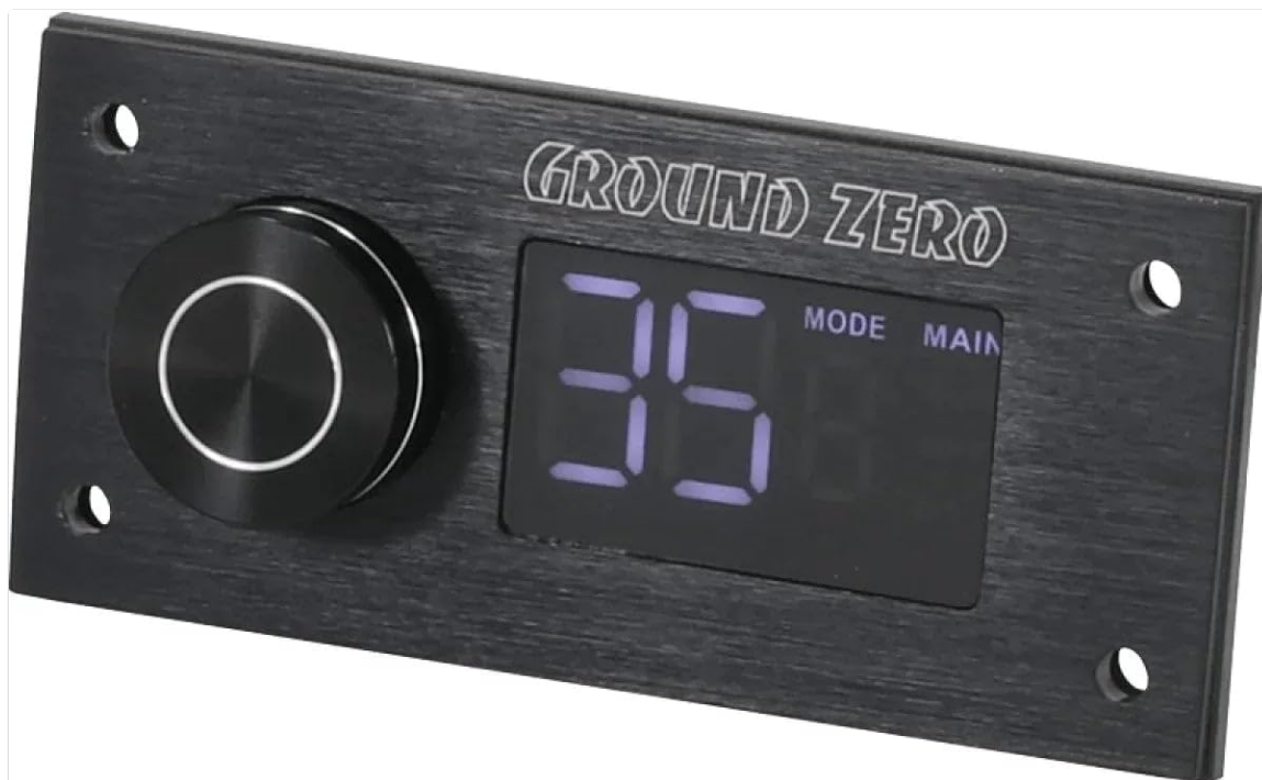
The GZDSP Remote PRO Control unit with its display and rotary knob.
