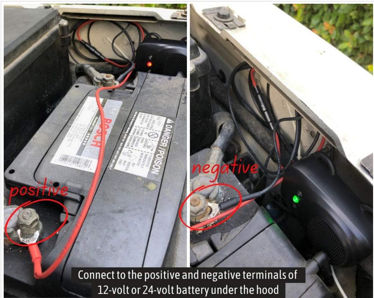
Image: Close-up view of the repellent connected to the 12-volt or 24-volt battery terminals under the hood.
