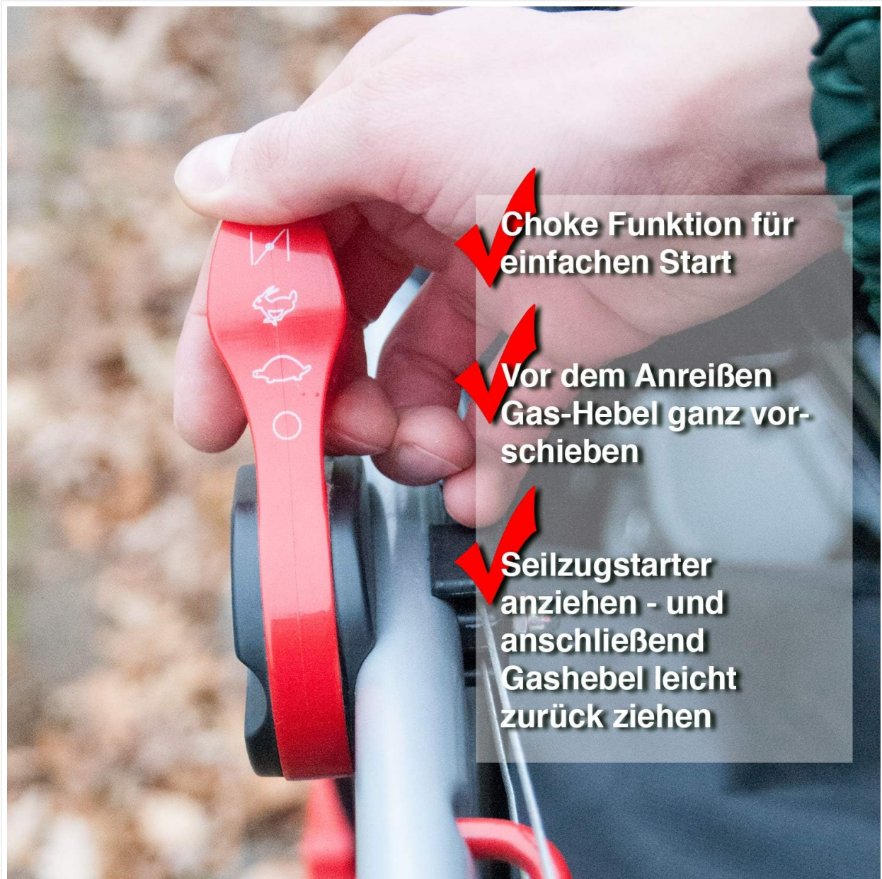
Figure 4: Illustration of the choke function for easy starting. Push the throttle lever forward, pull the recoil starter, then slightly pull back the throttle lever.
