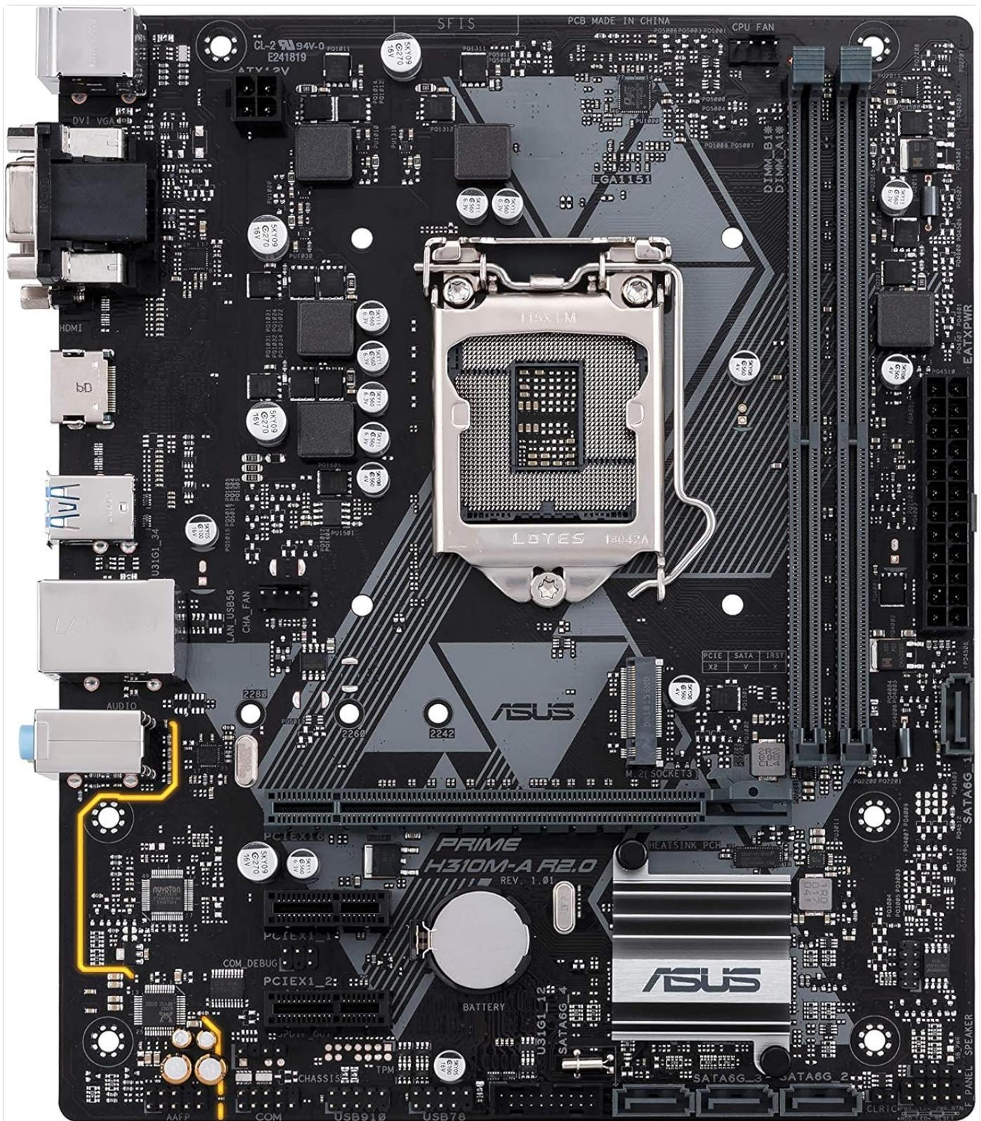
Figure 3.1: Top-down view of the motherboard, highlighting key component locations such as the CPU socket, DIMM slots, and PCIe slots.
