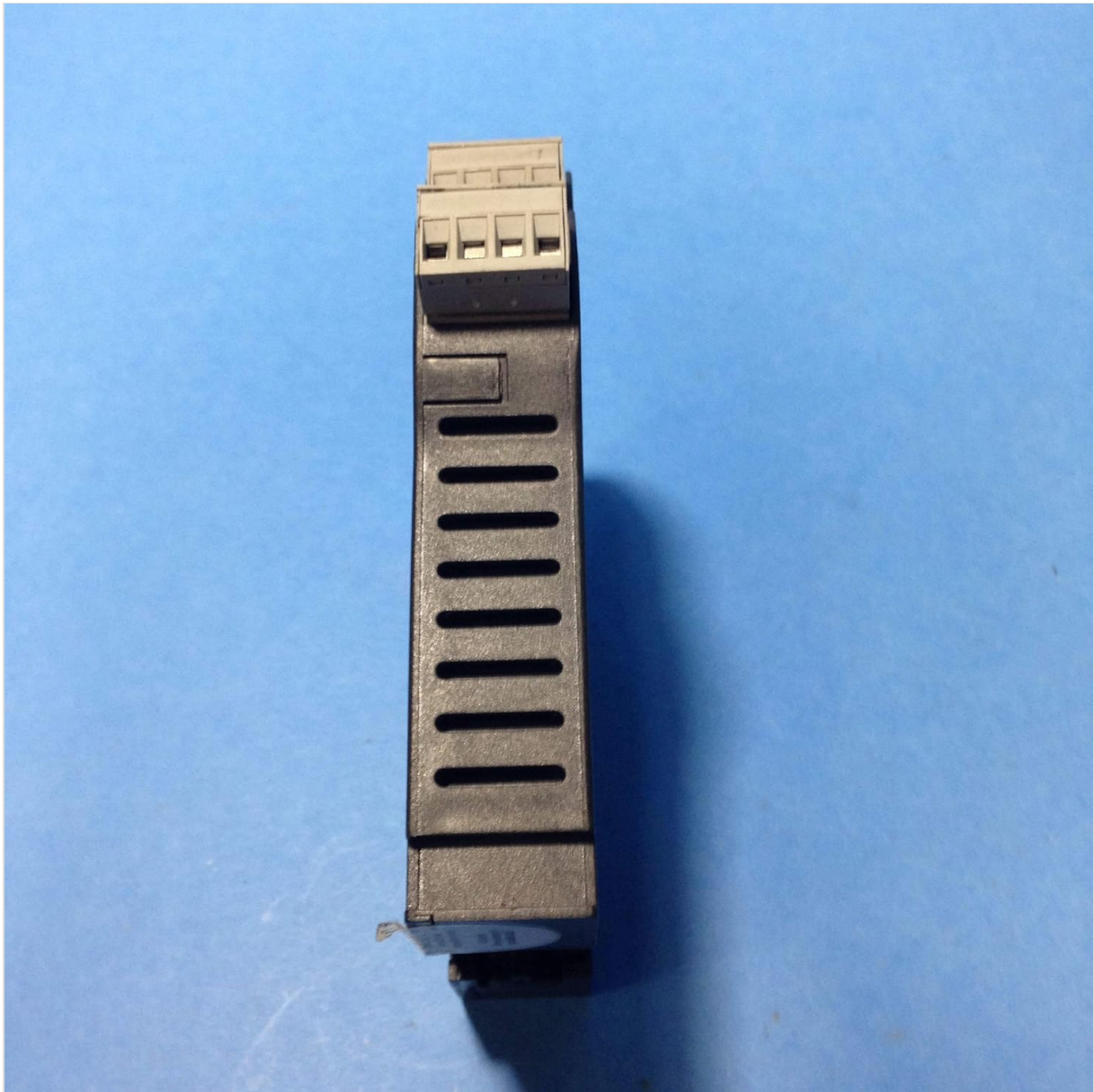
Figure 2: Side view of the Schmersal SRB 301AN-24V Safety Relay, illustrating its compact form factor suitable for DIN rail mounting.
