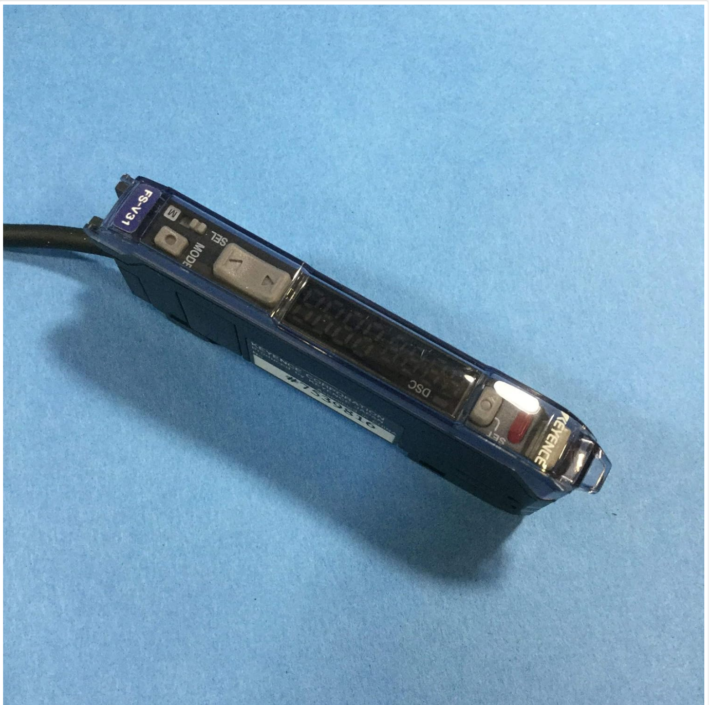
Figure 3.3: Keyence FS-V31 Control Panel. A detailed view of the sensor's control interface, highlighting the 'SEL' (Select), 'MODE', 'SET', and 'DSC' buttons, which are used for configuration and adjustment.
