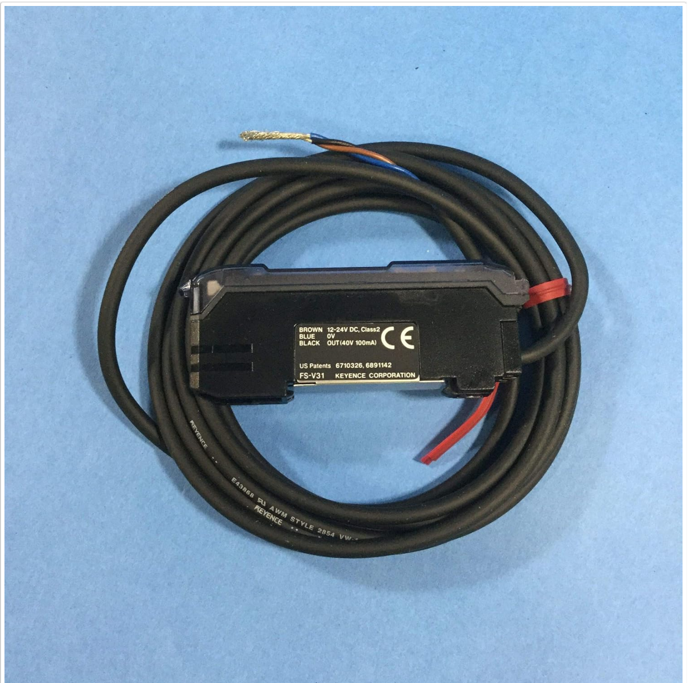
Figure 3.2: Keyence FS-V31 Wiring Details. This image provides a closer view of the sensor's wiring, indicating the color codes for power (BROWN, BLUE) and output (BLACK), along with the CE compliance mark.
