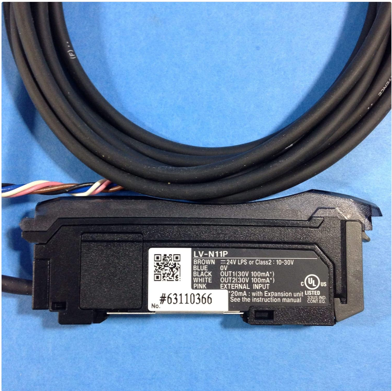
Image: Close-up of the LV-N11P label, detailing wiring connections and basic specifications.
